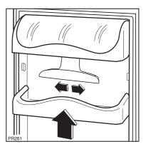
For more thorough cleaning, the top door shelf can be removed by pulling it in the direction of the arrows, then refitting it in position.
